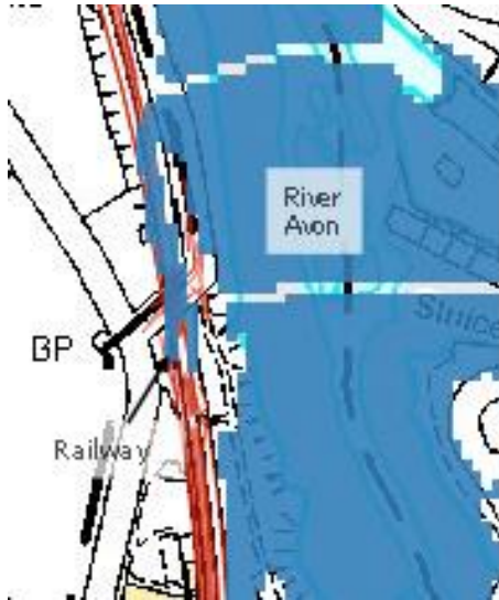
Figure 5. Flooding of the railway at chainage 6300
